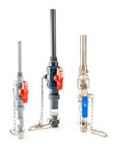
Griffco corporation stops (corp stops) are designed to ensure that chemical feed systems inject into the center of a process stream for better mixing and to prevent corrosion along the process pipe. They are also retractable and offer a ball valve to seal the process stream for servicing. Corporation stops are typically used for larger diameter pipe to inject chemicals away from the edge of the pipe. This allows for bet-
