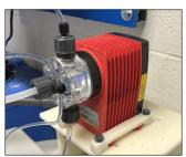
The Lutz-Jesco dosing head ventilation V stands for trouble-free dosing of outgassing chemicals and oxidizers like bromine, sodium hypochlorite (bleach), hydrogen peroxide, and more. An automatic vent valve sepa-
