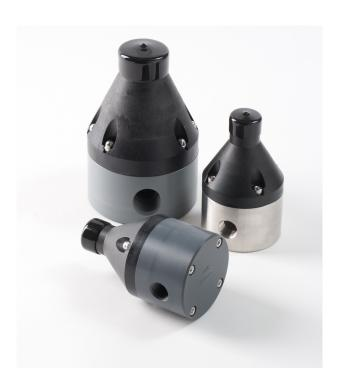
**Griffco** high flow diaphragm pressure relief valves are designed to protect chemical transfer systems from over pressure damage caused by defective equipment or a blockage in the chemical line. Large orifice sizes facilitate high flows and high viscosity. Wetted materials include: **PVC, CPVC, PP, PVDF, PTFE, 316 SS, A 20 and Hast. C.** Available in 1/2" – 2" sizes.
