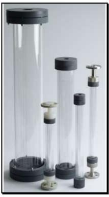
Griffco Borosilicate Glass Calibration Cylinders are designed to enhance the performance of chemical feed systems by providing a verification of the flow rate of the chemical feed pump. Constructed of borosilicate glass and a choice of 8 end cap materials, (PVC, CPVC, PP, PTFE, PVDF, 316SS, Alloy 20, and Hastelloy C) these cylinders are suitable for use with most chemicals. Available in 12 sizes; from 30mL to 20 L.
