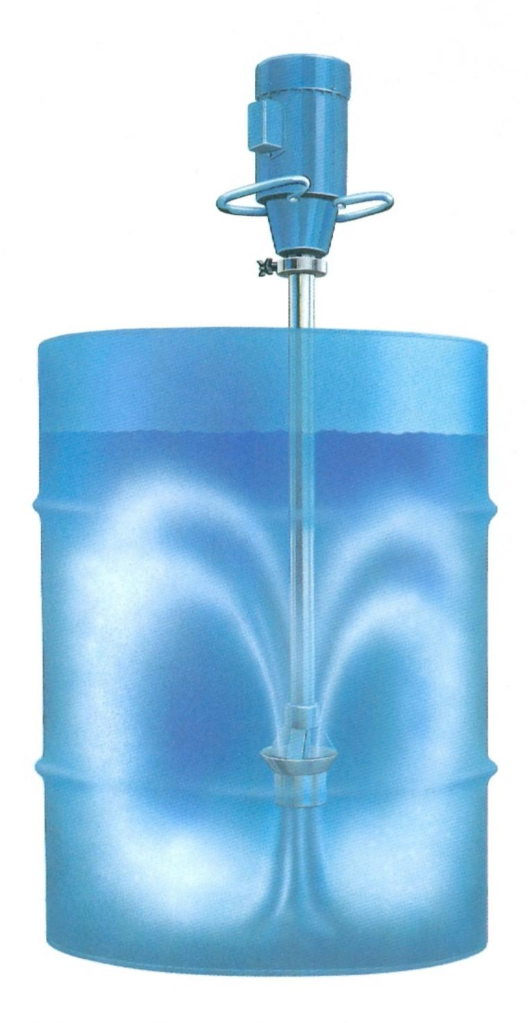
The all 316SS Jet Stream utilizes a stator and rotor combination for complete liquid mixing. All the liquid is pumped down by the rotor and through our patented stator. The material exits the stator in strong vertical lines to the bottom of the vessel. It is deflected sideways, passes up along the walls of the vessel guaranteeing a 100% homogenous mixture.
