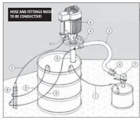
\*Zone "0": Defines a constant hazardous explosive atmosphere. Covers interior of drum/container used for storing or transporting of explosive liquids. Equipment approved for zone "0" must be specially tested and certified.
