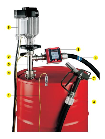
Bonding is the electrical interconnection between containers (such as drum and a receiving can). Bonding must be completed before pumping begins. For better conductivity paint and dirt shall be removed from the contact points.
