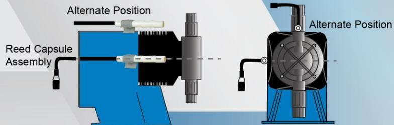
Operation can be verified by a simple electrical continuity check between the plug terminals. The reed switch is normally open, and closes in the presence of a magnetic field of sufficient strength. This can be verified with the capsule in place on an operating transmitting pump (each pump stroke causes momentary closure) or, on the bench, by positioning a small permanent magnet next to the capsule (which causes closure). The assembly is not repairable and must be replaced as a unit.
