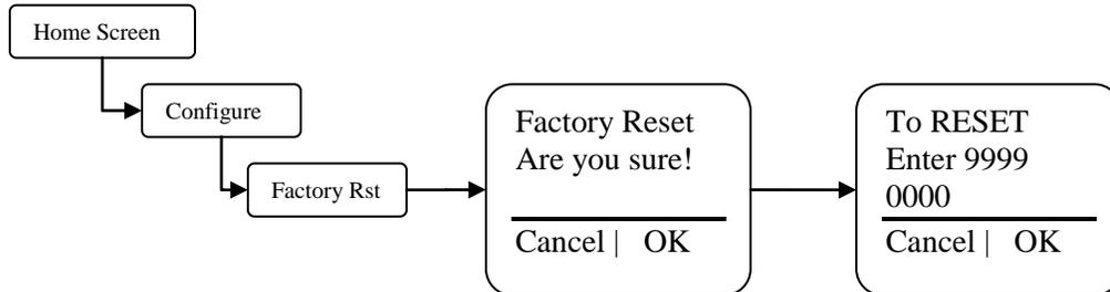
Use this function to reset the controller back to the factory defaults.
