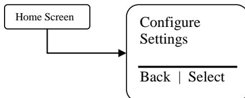
**Configure** – This menu allows you to set the time and date, display contrast, water meter, etc.
