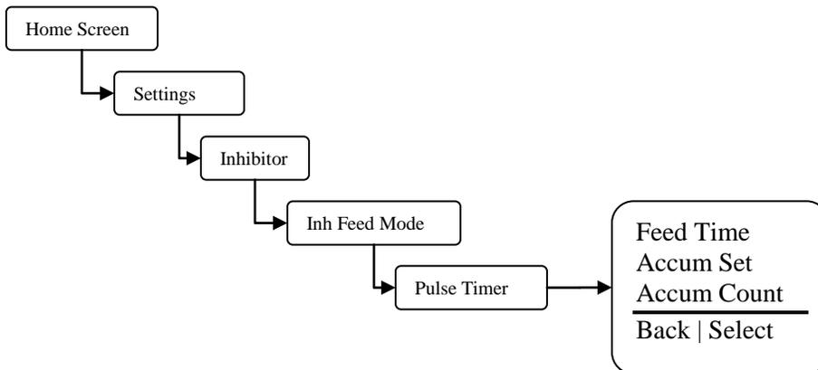
**Feed Time** – Set this value to the amount of time you want the inhibitor to feed when the water meter accumulator reaches its target.
