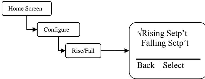
**Rising Setpoint** – Select this option if a cooling tower is being controlled.
