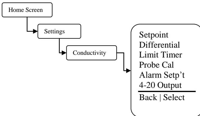
**Setpoint** – Set the conductivity setpoint. This is the conductivity point where a bleed function will begin. Once the conductivity has reached this value the bleed function will begin.
