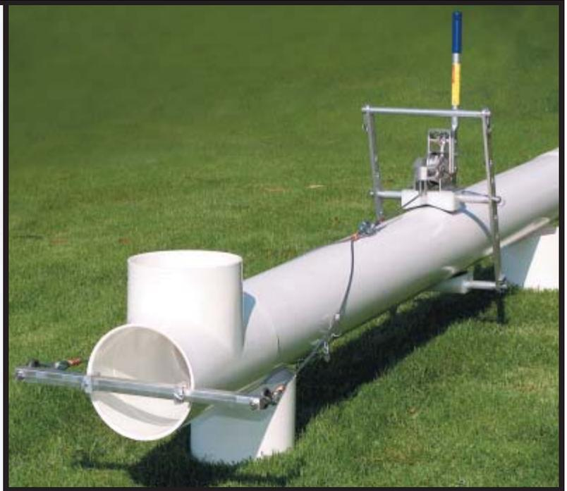
**Not only does the pipe puller make the perfect joint, it reduces installation time.**
